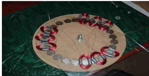
*Fig.6 Magnet placing on stator*
